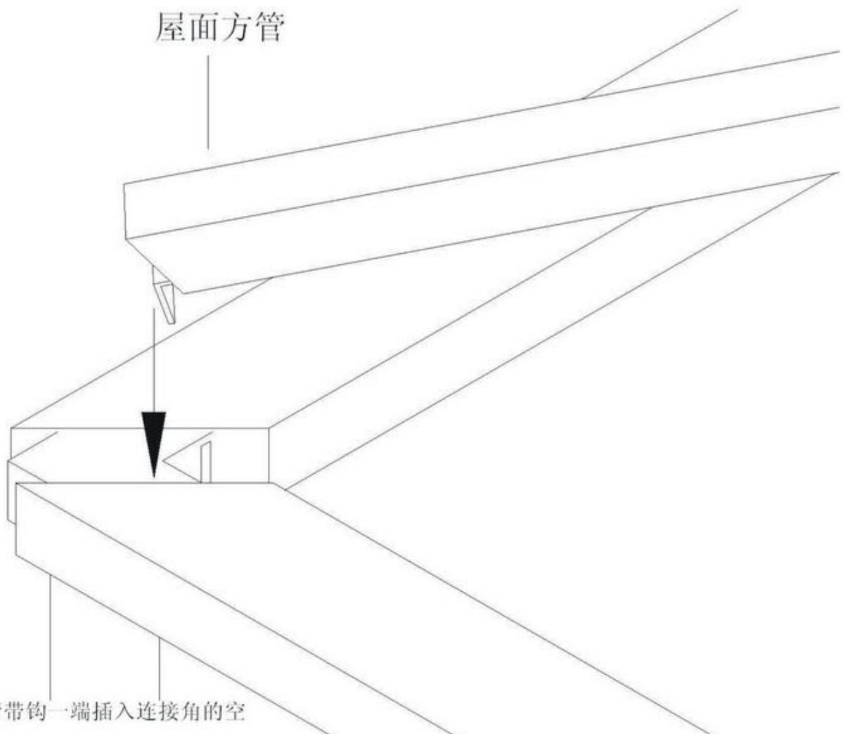
**Put one end of hook of the roofing square pipe into the empty of connection triangle.**
